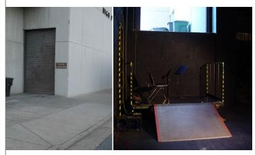
**Loading Dock:** The dock is 39" high and leads directly to the freight elevator. The Rollup Door's ramp is also a dock plate. Freight elevator is 8'6" long x 6' wide x 7' tall. Elevator doors are 6'2" tall x 4'6" wide. Elevator access to Stage level, Dressing rooms, Front of House, and Balcony/Booth levels.
